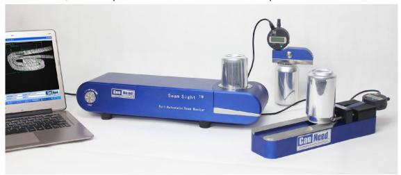
Without cutting or destructing the sample cans, the "CanNeed-STG-200-d Seam Thickness Gauge (Digital)", "CanNeed-SLG-d Seam Length Gauge" and "CanNeed-CSG-200S Countersink Gauge (Digital)" compose the quick measurement tools for double seam quality control.
