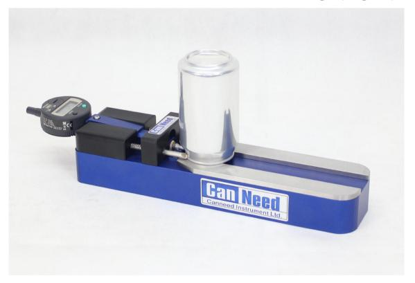
After the double seam structure was cut, the seam thickness that measured on the seam monitor is not accurate, therefore, seam thickness need to be measured before the double seam structure was cut.
