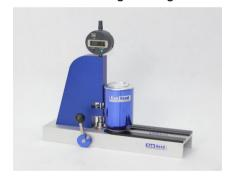
CanNeed-SLG-d Seam length gauge is used to measure the Seam length (Seam height)
