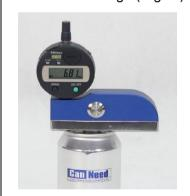
CanNeed-CSG-200S Countersink Gauge (digital) is used to measure the Countersink depth.
